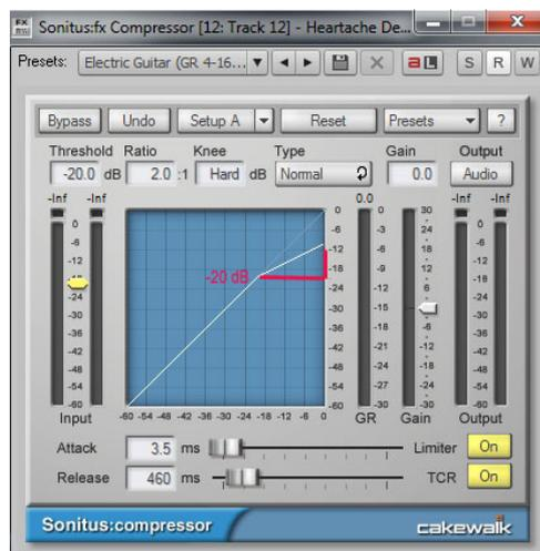
In this case we have a ratio of 2.0 to 1, and that is shown in the parameters above the top LHS of the graph. This would have the effect of reducing how much the volume of the signal changed by, and limiting the output signal to a maximum of -10 dB.
