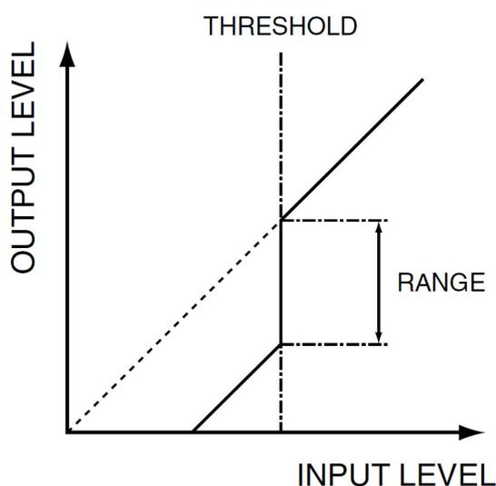
The Range is the amount the output has been reduced by, and this is user adjustable as well as the threshold.
