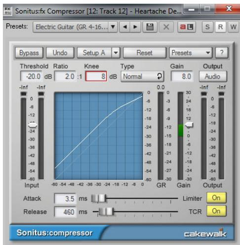
**The Knee** – This controls the behavior of the compressor around the threshold level. The knee shown above is a hard knee, meaning that the changes applied to signal level are applied fully, once the incoming level exceeds the threshold.
