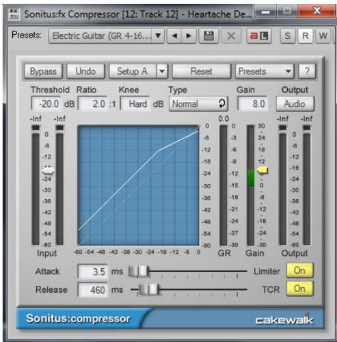
This will have the effect of boosting the signal level when it is soft, but reducing the changes of level when it starts to get loud, and always keeping it below a potential distortion point, particularly in the digital recording world.
